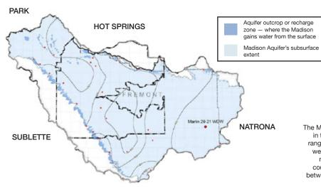
The Madison Aquifer abuts granite formations in the Wind River and Owl Creek Mountain ranges. Waste injected into the Marlin 29-21 well, pictured, could flow through fractures many miles from this injection point, and could move upward at the point of contact between the aquifer and adjacent formations (the dark blue areas pictured).
